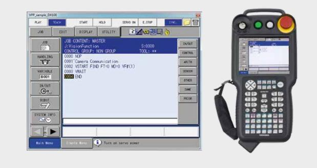
This function is an inform instruction to communicate with different Vision System. It maps the communication protocols of a variety of selected vision systems and works, dependent on these, on the basis of Ethernet or RS232. This robot instruction allows easy control of image processing devices.
