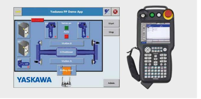
The "Advanced PP Customization Runtime" is required to run applications developed with "Advanced PP Customization" SDK. The SDK is a collection of modules for creating customized user interfaces for the programming pendant. The customized UI overlies the standard UI so it's possible to make important controls and informations easier to reach and create a unique interface concept across multiple devices.
