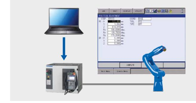
The "Teaching Point Adjustment" function modifies the taught position data by entering the numeric number on the programming pendant without operating the manipulator.
