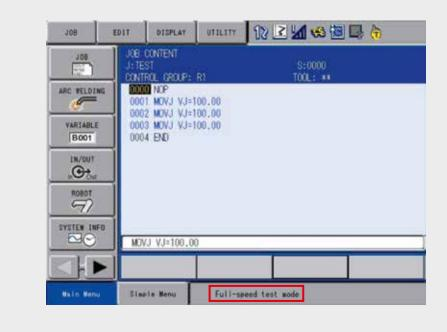
This signal is used to reset the slow speed limit for the test run in the teach mode.
