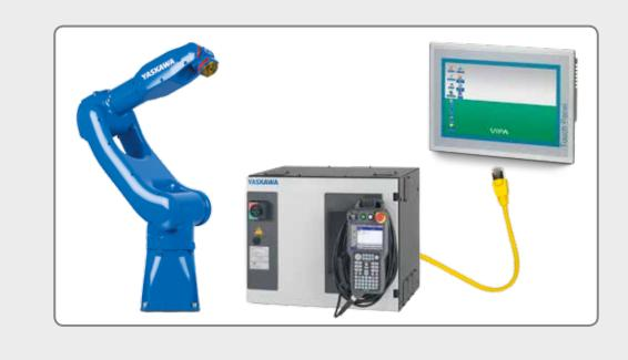
With "MOTOModbus", YASKAWA opens up a standard interface to almost any HMI (Human-Machine Interface = connection/hardware between human and machine).
