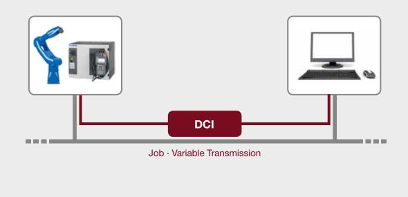
The "Data Transmission" function (DCI) allows to load and save jobs and variables from inform by using DCI commands.
